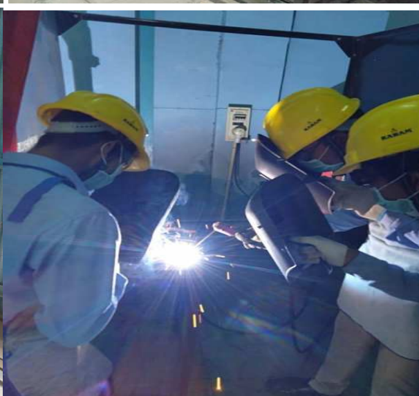
Day 3: Cutting of workpiece using grinder and Preparing V butt by welding
